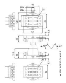
· Instruction to fix the knife-switch on structures
