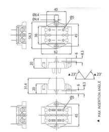
· Instructions to fix the knife-switch on structures
